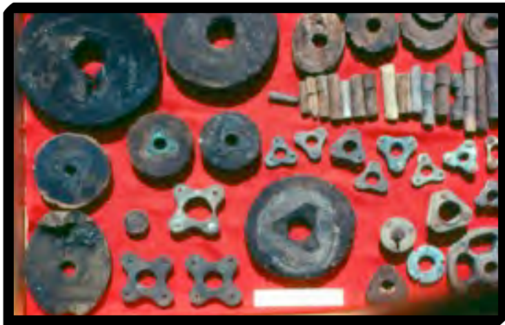
Assemblage of sheaves and pins from underwater in English Harbour. The three point versions are older than the four pin variety.
