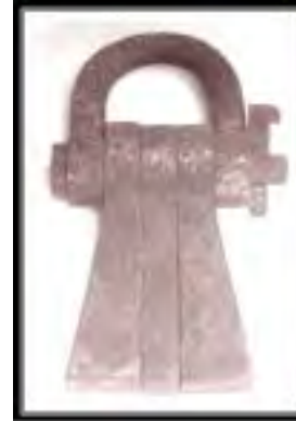
This tool known as a Lewis fitted into the dovetail cut in the rock. It could then be lifted.
